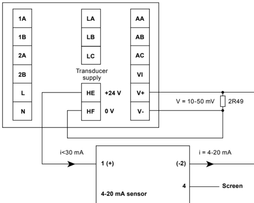
Wiring diagram for connecting the transmitter SX90
