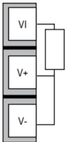
The resistance of the tree wires must be the same. The line resistance may cause errors if it exceeds 22  $\Omega$ .
